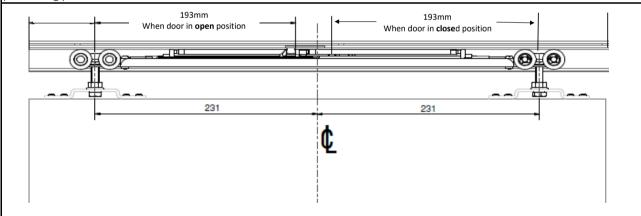
**STEP 8:** Centre the door and insert the triggers at either side into the correct position, securing into place with an allen key. The marks you created on the track in step 7 should line up exactly with the protruding part of the trigger.
